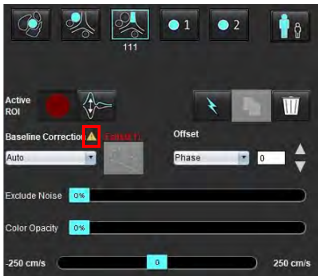
FIGURE 6. Baseline Correction Failure
