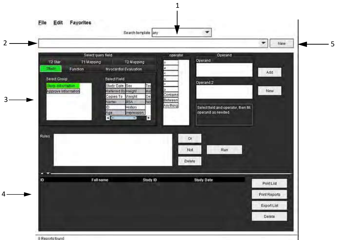
1. Search template drop-down menu, 2. History bar, 3. Create query fields, 4. Query results, 5. New button
